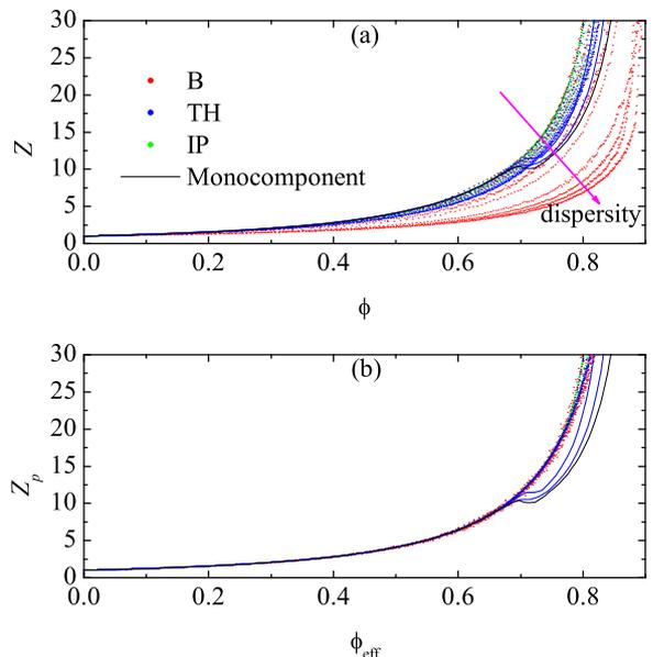
Figure 1: (a) Bare simulation values for different HD mixtures. (b) Inference of the EoS for the monocomponent fluid.
