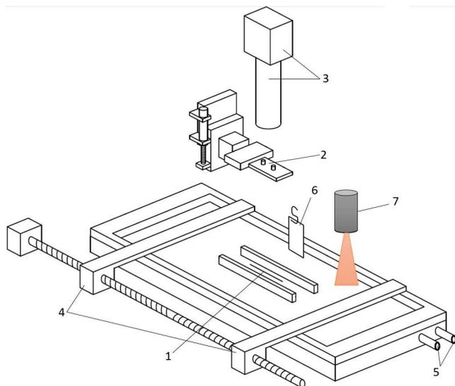
Figure 1: Schematics of the interfacial shear rheometer comprising the following elements: (1) magnetic probe, (2) magnetic tweezers, (3) optical inspection system, (4) mobile barriers, (5) thermostatic bath, (6) surface pressure sensor, and (7) infrared sensor.
