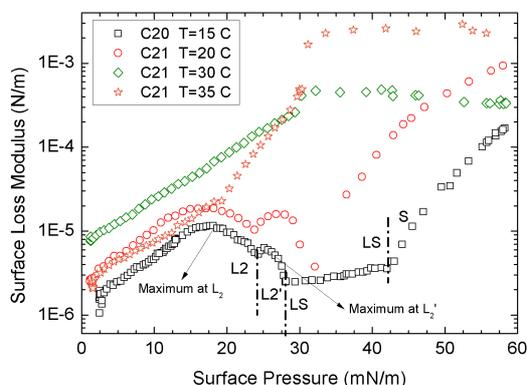
Figure 2: Surface loss moduli versus surface pressure for different fatty acids and temperatures.
