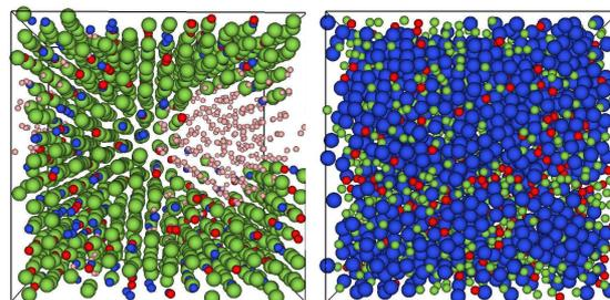
Figure 1: System state under shear by MD-DPD method to show as the structure changes in the solid-solid transition: liquid (pink), bcc(green), hcp(red) and fcc(blue) particles. A smaller radio is used to emphasize the predominant crystal structures *Left*: First step with bcc-like order; *Right*: Second step with fcc-like order.
