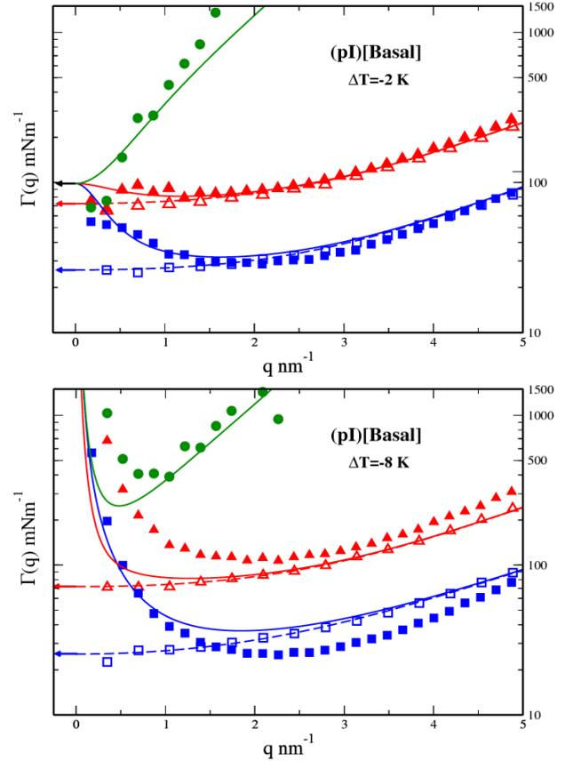
Figure 1: Observation of a roughening transition on the prismatic surface of ice. At a temperature 2 K below the triple point, the wave-vector dependent components of the stiffness tensor converge to a finite value at  $q \rightarrow 0$  that is the sum of the ice/water and water/vapor stiffness coefficients. Six Kelvin below, the stiffness coefficients diverge, indicating the onset of a smooth facet.
