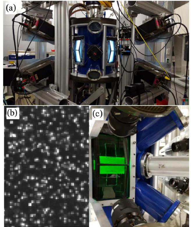
Figure 1: (a) Experimental setup with tank and 4 cameras. (b) Cut-out of a typical particle image at moderate seeding density. (c) Close-up of camera lenses, prisms, and illuminated volume with particles.
