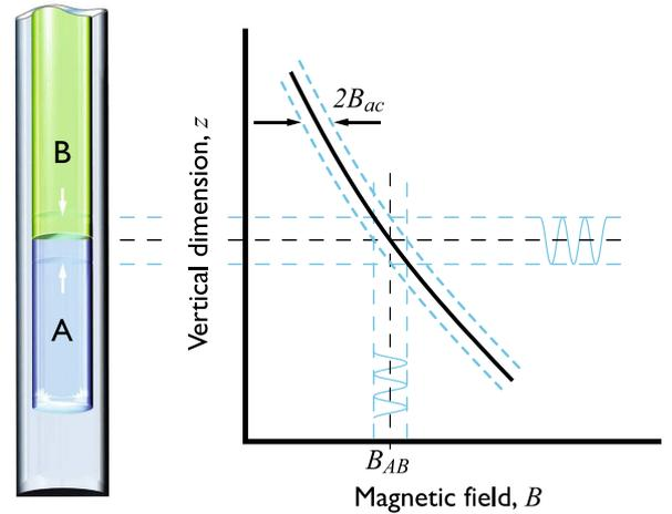
Figure 1: The bottom end of the sapphire black body radiator contains A phase in the bottom and B phase in the top. The A-B interface is stabilised at a position  $z_{eq}$  corresponding to the transition field  $B_c$  by a shaped magnetic field profile (solid line) provided by the solenoid stack. Oscillating the field profile oscillates the equilibrium position  $z_{eq}$  along the cell axis. The oscillatory response of the A-B interface depends on its effective mass and friction.
