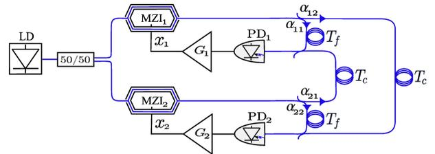
Figure 1: Diagram of the system modeled. Each OEO consists of a Mach-Zehnder interferometer (MZI), a fiber loop with delay  $T_f$ , a photodiode (PD) and a RF amplifier (G) whose output modulates an MZI arm. OEOs are fed by a laser diode (LD) and are mutually coupled with delay  $T_c$ .
